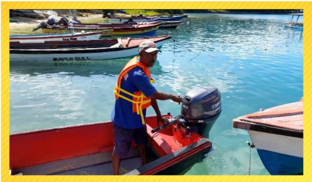
Figure 9: A warden of the Orcabessa Marine Trust demonstrates the pollution free, quiet operation of the newly installed 4-stroke engine on the sanctuary's patrol boat
